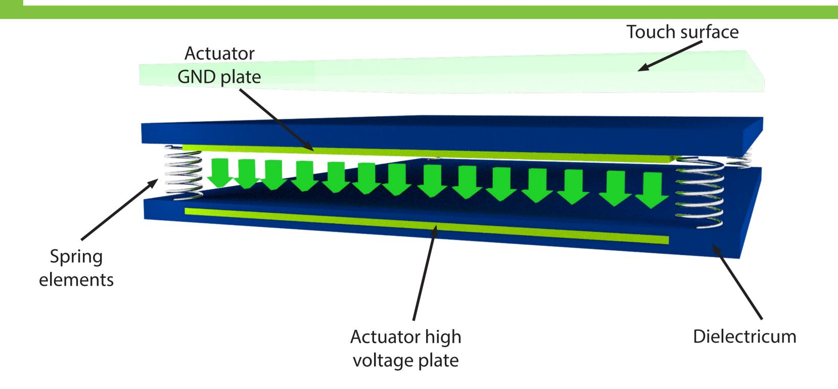
Based on electrostatic principle, we offer solutions that allow you to feel the UI elements, before they are actually activated.
